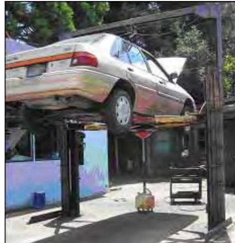
This small auto repair shop performs work outdoors without a roof and without berms or other containment for spills, which increases the threat of stormwater pollution.
